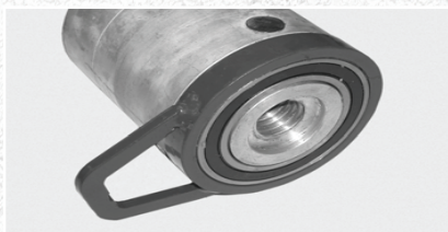
Install pulling eye bearing on wall plug.
