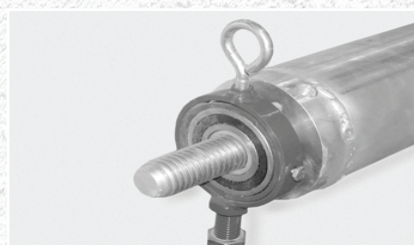
Remove pivot bearing from the centering tube and install on the UHMW bushing.
