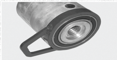
Install pulling eye bearing on wall plug.
